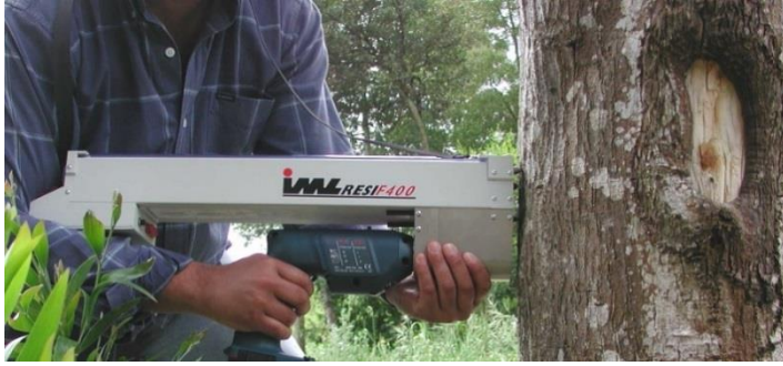
Resistance-recording drill, Image from: arvores-e-pessoas.pt
