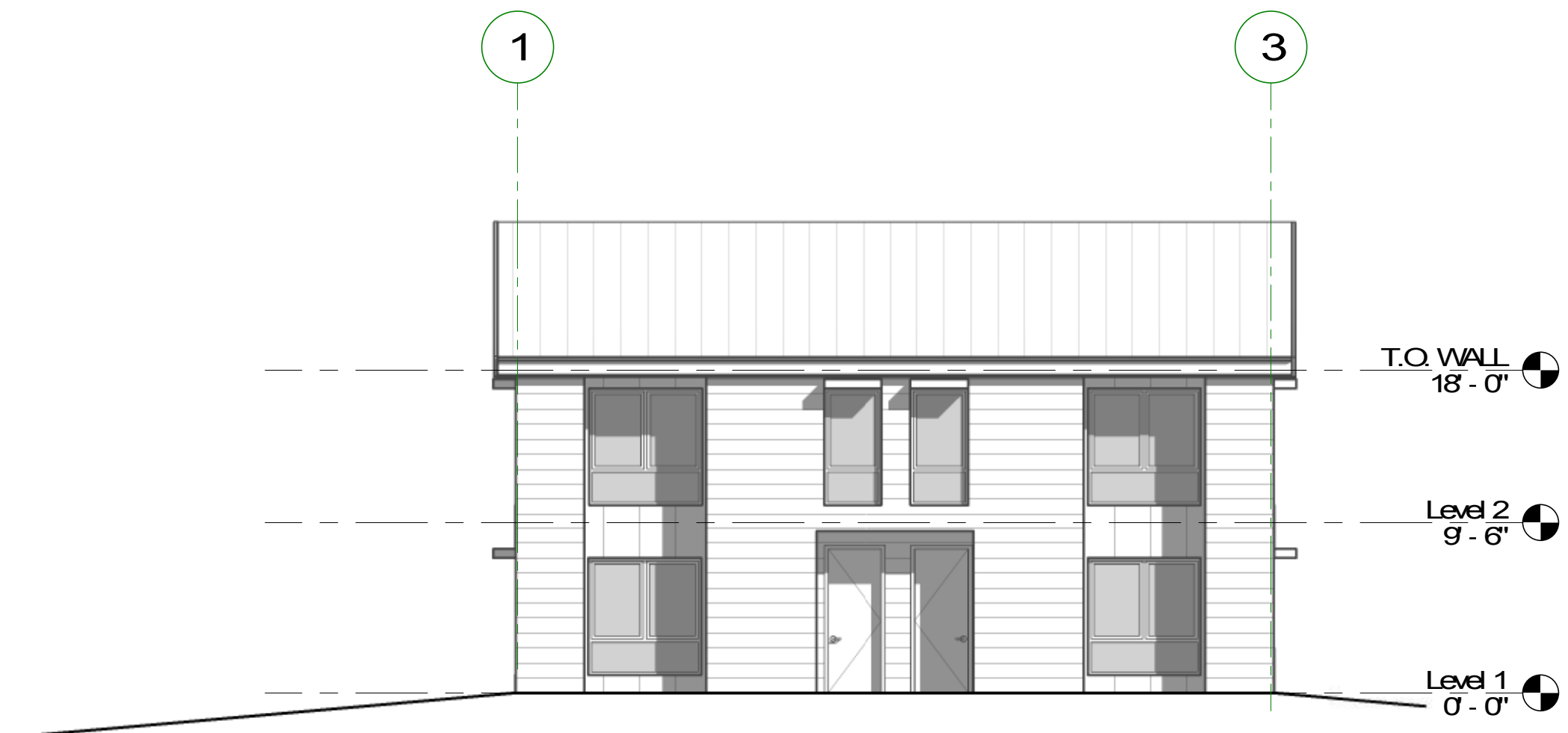
BLDG TYPE A - SOUTH ELEVATION 1/8" = 1'-0" 5
