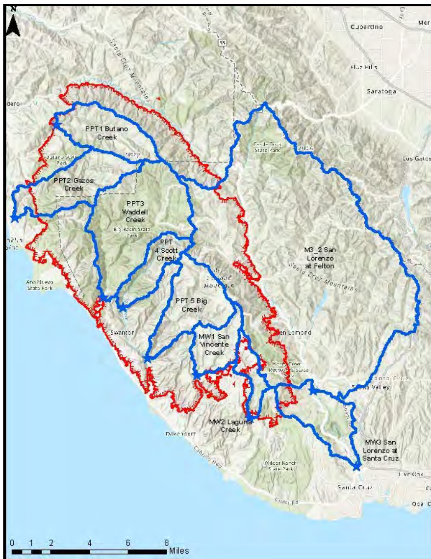
Figure 8. Pour point watersheds for the CZU Lightning Complex. Post-fire peak flows were estimated for Butano, Gazos, Waddell, Scott, and Big Creek. Proportion of watershed area by soil burn severity was extracted for San Vicente Creek, Laguna Creek, and the San Lorenzo River at two locations to inform threats to municipal water supply.
